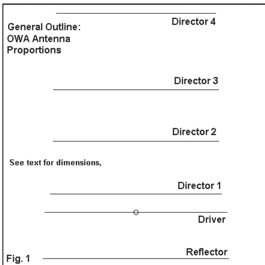
The 20-meter antenna has several features that deserve special note. Director 1 is perhaps the most significant, since it represents the added element to previously standard 5-element designs. By the use of this parasitic element, the driver can be more closely spaced to the reflector and still show a feedpoint impedance very close to 50 Ohms resistive. Moreover, the antenna shows wideband VSWR characteristics, with values less than a 1.3:1 from 14.0 through 14.35 MHz.
