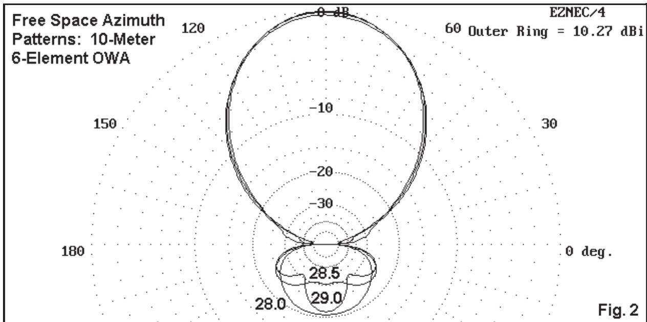
The antenna pattern itself is a model of good behavior, with no undesirable side or rear lobes. Note in **Fig. 2** the change in the shape of the rearward lobe across the band, which is a normal progression for well-behaved antennas of this type.
